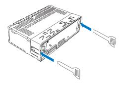
3 Install the sleeve into the dashboard and bend the tabs outward to fix the sleeve.
