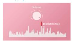
Anti-Clipping lets you play music louder and keeps it high quality, even when the battery is low. It accepts a range of input signals, from 300mV to 1000mV and keeps your speakers safe from damage by distortion. This built-in function monitors the musical signal as it goes through the amplifier and keeps peaks within the amplifier's range, preventing the audio distortion caused by clipping without affecting loudness. A portable speaker's ability to reproduce musical peaks decreases along with
