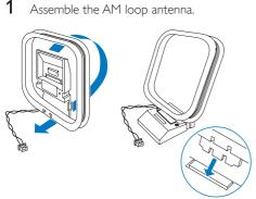
2 Connect the AM loop antenna to the AM jack on the back of the main unit. Adjust the position of the antenna for optimal reception.
