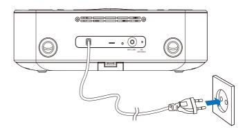
1 Connect the AC power cord to the wall outlet.
