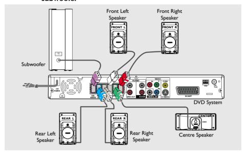
Connect the supplied speakers system using the fixed speaker cables by matching the colours of the sockets and speaker cables.
