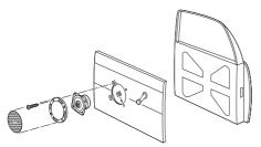
**8** Press and insert the edges of the grille net.
