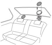
Follow the steps in section "Option 1: Mount in door" to mount the speakers into the rear tray.
