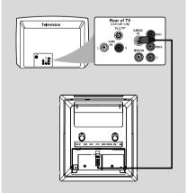
Use the S-Video cable (not supplied) to connect the system's S-VIDEO jack to the S-Video input jack (or labeled as Y/C or S-VHS) on the TV set.
