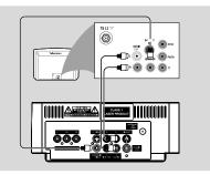
Use the supplied composite video cable (yellow) to connect the system's COMPOSITE
