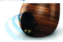
Bass-reflex acoustic load uses a bass pipe tuned to the acoustic volume of the speaker box, in order to reproduce deep bass from compact enclosures. The carefully designed profiled bass-pipe helps air flow and allows for deep and impactful bass, even at loud volumes while minimising air turbulence that may cause distortion.
