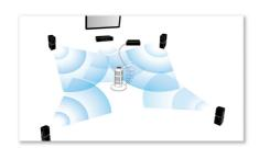
Adjusting your new Philips home theatre for optimum sound experience is now a breeze. With the simple touch of a button on the remote, the intelligent pre-loaded sound calibrator software is launched and emits test signals to the speakers. These signals are captured and analysed by the auto-calibration microphone and the necessary adjustments are made, taking into consideration the distances between speakers and listening positions, the loudness and the delay response of audio
