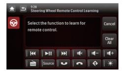
4 Tap an icon, for example, I◄◀, of which you want to assign the function to a button on the steering wheel.
