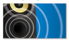
Bass Reflex Speaker System delivers a deep bass experience from a compact loudspeaker box system. It differs from a conventional loudspeaker box system in the addition of a bass pipe that is
