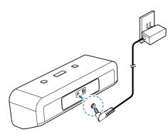
Connect the AC power adaptor, one end to the power socket on the back of the unit, and the other the wall power supply.
