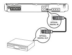
1 Connect an optical cable (not supplied) to the OPTICAL DIGITAL-IN jack on the Home Theater System and the OPTICAL/SPDIF output jack on the device.
