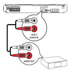
Connect the audio cables (not supplied) to the AUDIO IN-AUX2 jacks on the Home Theater System and the AUDIO output jacks on the device.
