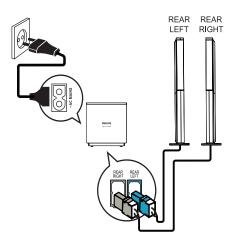
1 Connect the rear left and right speakers to the matching jacks at the bottom of the wireless receiver.
