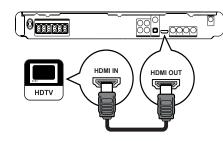
1 Connect an HDMI cable (not supplied) to the HDMI OUT jack on this Home Theater System and the HDMI input jack on the TV
