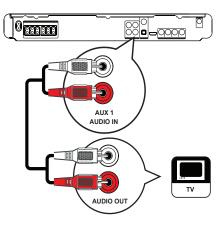
Connect the audio cables (not supplied) to the AUDIO IN-AUX1 jacks on the Home Theater System and the AUDIO output jacks on the TV.
