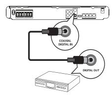
1 Connect a coaxial cable (not supplied) to the COAXIAL DIGITAL-IN jack on the Home Theater System and the COAXIAL/DIGITAL output jack on the device.
