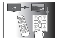
5 You can press STOP to confirm and exit the search. If most of the other keys does not work properly, turn off your TV and press PLAY again to try the next code.
