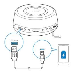
2 Connect the alarm clock to power. → Once the device is recognized, the charging starts.
