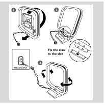
Position the antenna as far as possible from a TV, VCR or other radiation source. It is unnecessary to connect the FM pigital antenna since it is fixed to the main unit..
