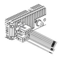
2 Check the car's wiring carefully and connect them to the ISO connector.
