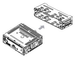
5 Install the sleeve into the dashboard and bend the tabs outward to fix the sleeve.
