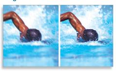
resolution of the image resulting in a noticeably sharper picture. Instead of sending a field comprising the odd lines to the screen first, followed by the field with the even lines, both fields are written at one time. A full image is created instantaneously, using the maximum resolution. At such a speed, your eye perceives a sharper picture with no line structure.
