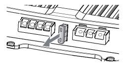
If the fuse gets damaged immediately after it has been replaced, the amplifier might have internal malfunction. Consult qualified personal for repair:
