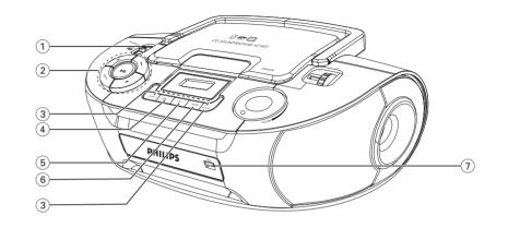
1. Source selector Slide to select function: CD/MP3. USB. AUX or radio
