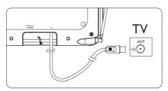
2 Connect the DC plug to the antenna and the power supply to a 100-240V AC outlet.
