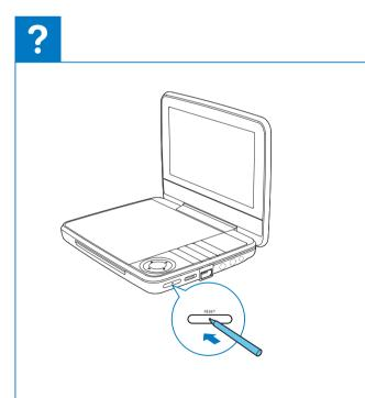
If the player does not respond to key pressing, press **RESET** with a ball-point pen or similar tool to switch off the player, and then press ① to restart.
