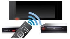
EasyLink lets you control multiple devices like DVD players, Blu-ray players, soundbar speakers, Home theatre systems and TVs etc. with one remote. It uses HDMI CEC industrystandard protocol to share functionality between devices through the HDMI cable. With one touch of a button, you can operate all your connected HDMI CEC-enabled equipment simultaneously. Functions like standby and play can now be carried out with absolute ease.
