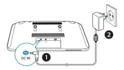
Connect the power cable to the wall socket.
