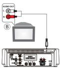
(B) To listen to TV through this system, use a cinch cable (not supplied) to connect AUX IN jack (3.5mm) to the corresponding AUDIO OUT jacks on the TV set.
