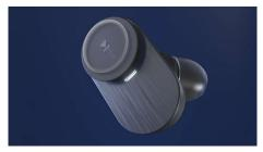
Touch controls keep things simple, and Bluetooth multipoint lets you connect to a phone (iOS or Android) and laptop at the same time. Google Fast Pair lets you pair to a compatible Android device with a single tap.
