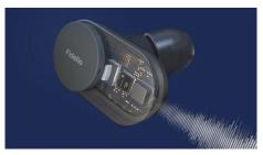
Multiple mics and a dedicated algorithm focus on the sound of your voice as well as reducing noise from the world around you. Even wind noise is filtered out, so you can be heard clearly when on a call outside.
