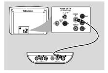
Use an S-Video cable (not supplied) to connect the S-VIDEO OUT jack to the S-Video input jack (or labeled as Y/C or S-VHS) on the TV.
