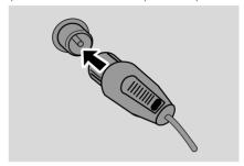
For better FM stereo reception, connect an outdoor FM antenna to the FM AERIAL (FM ANTENNA) terminal.
