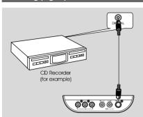
Connect the COAXIAL (DIGITAL OUTPUT) jack on the video box to the DIGITAL IN jack on a digital recording device (such as DTS Digital Theatre compatible, with Dolby Digital decoder).
