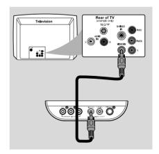
Use a composite video cable (yellow-not supplied) to connect the VIDEO OUT jack on the video box to the video input jack (or labeled as A/V In, CVBS, Composite or Baseband) on the TV.
