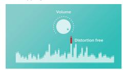
Anti-Clipping lets you play music louder and keeps the quality high, even when the battery is low. It accepts a range of input signals from 300 mV to 1000 mV and keeps your speakers safe from damage by distortion. This built-in function monitors the musical signal as it goes through the amplifier and keeps peaks within the amplifier's range, preventing the audio distortion caused by clipping without affecting loudness. A portable speaker's ability to reproduce musical peaks decreases along with
