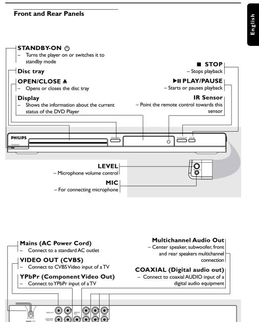
Caution: Do not touch the inner pins of the jacks on the rear panel. Electrostatic discharge may cause permanent damage to the unit.
