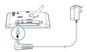
2 Connect the power cord to a power supply socket.
