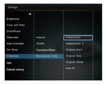
→ If you select [RadiantColor], the PhotoFrame extends the color on the edges of a photo that is smaller than the full screen to fill the screen without black bars or aspect ratio distortion.
