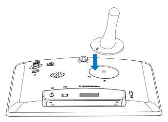
2 Turn the stand anti-clockwise 45 degrees to the \( \Delta \) position and lock it to the PhotoFrame firmly.
