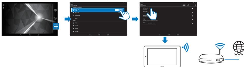
**EN** Through Wi-Fi, connect PI3105 to the Internet. On the pop-up screen for setup options, drag the slider to switch on Wi-Fi and connect to an available network.
