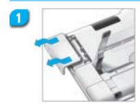
Open the Wireless LAN Adapter cover by pushing in the grips and sliding off the cover in the indicated direction.
