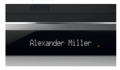
The Philips Monolith high contrast white-onblack display seamlessly and stylishly integrates with its base. The display shows the caller ID when there is an incoming call and the time when in idle mode. You can choose to turn off the base display - so as not to be disturbed by any light - at any time.
