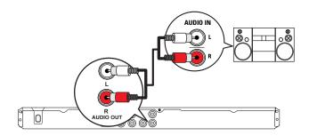
1 Connect the audio cables (supplied) to the AUDIO OUT L/R jacks on this DVD player and the audio input jacks on the device.
