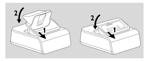
To connect with a different iPod/GoGear portable player, pop up the corresponding dock adapter and replace with a new one of the matching type.
