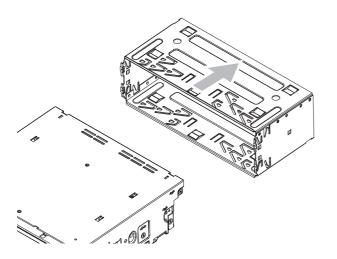
5 Install the sleeve into the dashboard and bend the tabs outward to fix the sleeve.
