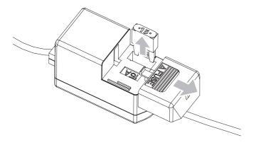
If the fuse gets damaged immediately after it has been replaced, there may be an internal malfunction. In such case, consult your Philips dealer.
