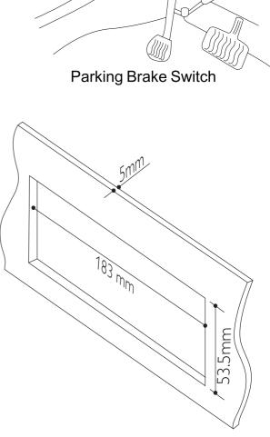
• Since the unit cannot be used if the dashboard opening's slant angle is above 20 degrees: Ensure that the horizontal slant of the car dashboard opening is between 0 and 20 degrees
