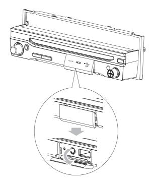
2 Insert the USB device or SD/MMC card into the USB socket or SD/MMC card slot.
