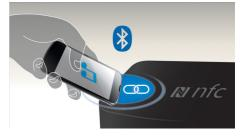
Pair Bluetooth devices easily with one-touch NFC (Near Field Communications) technology. Just tap the NFC enabled smartphone or tablet on the NFC area of a speaker to turn the speaker on, start Bluetooth pairing, and begin streaming music.
