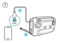
3 Slide the power source selector to CHARGE MOBILE. (Fig. (\*)
