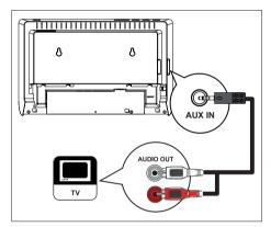
1 Connect an audio cable (supplied) from the AUX IN sockets on this unit to the AUDIO OUT sockets on your TV.
