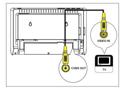
1 Connect a composite video cable (not supplied) from the CVBS OUT socket on this unit to the video input socket on your TV.
