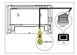
1 Connect the scart converter cable (supplied) from the CVBS OUT socket on this unit to the scart input socket on your TV.
