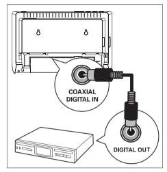
1 Connect a coaxial cable (not supplied) from the **DIGITAL IN-COAXIAL** socket on the subwoofer to the COAXIAL/DIGITAL OUT socket on the device.
