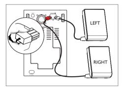
Connect the left and right speakers to the matching sockets on the subwoofer.
