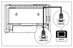
1 Connect a HDMI cable (not supplied) from the HDMI OUT on this unit to the HDMI IN socket on your TV.
