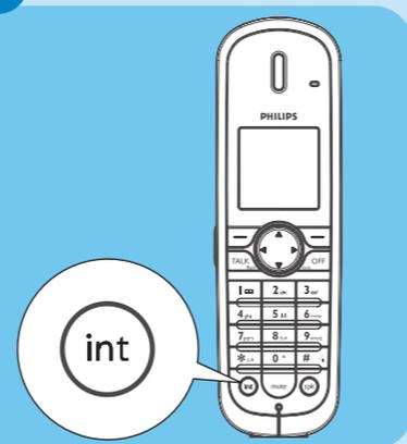
During a call in progress you can transfer the external call to a specific handset.
