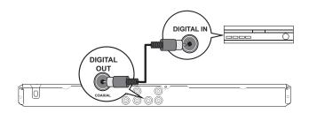
1 Connect a coaxial cable (not supplied) to the COAXIAL/DIGITAL OUT jack on this DVD player and the COAXIAL/DIGITAL input jack on the device.
