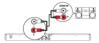
1 Connect the audio cables (supplied) to the AUDIO OUT L/R jacks on this DVD player and the audio input jacks on the device.
