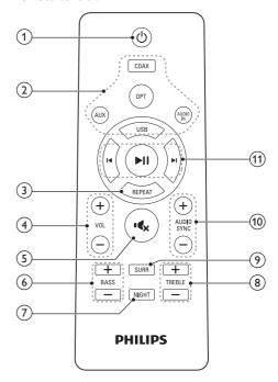
① ပံ (Standby-On) Switch the SoundBar on or to standby.
