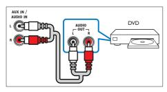
Using an analog cable, connect the AUX connectors on your SoundBar to the AUDIO OUT connectors on the TV or other device
