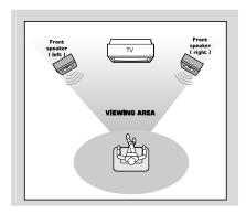
Place the front left and right speakers at equal distances from the TV set and at an angle of approximately 45 degrees from the listening position.
