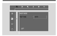
The system will start testing the speaker from left speaker to right speaker cyclically until you exit tone test
