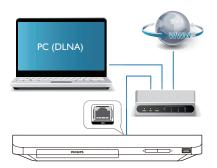
For Wi-Fi, connect a Philips Wi-Fi USB adapter (named WUB1110) to the ← (USB) connector on the front panel of this player.
