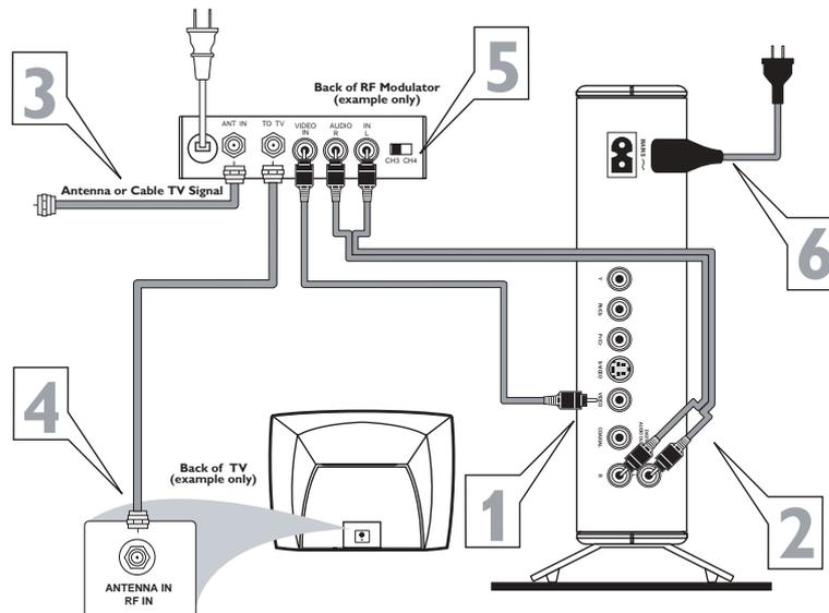
**Before you begin, make sure you have an RF modulator and extra RF coaxial cables. These are not supplied with the Player, but are available from Magnavox or most consumer electronics retailers.**
