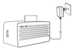
Connect the power adaptor to the AC power outlet.
