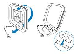
2 Connect the AM loop antenna to the AM jack on the back of the main unit. Adjust the position of the antenna for optimal reception.
