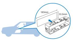
4 Bend the tabs outward to fix the sleeve.
