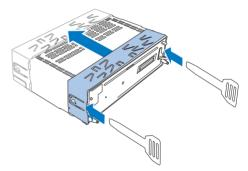
3 Install the sleeve into the dashboard.
