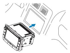
7 Fix the unit onto the dashboard with screws.
